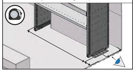
After ensuring the area under the floor bracket / vehicle floor is free from obstruction, mark the hole centres of the fixing slots. Move the unit to one side and drill Ø8.5mm through the floor of the vehicle (three positions for each bracket).
