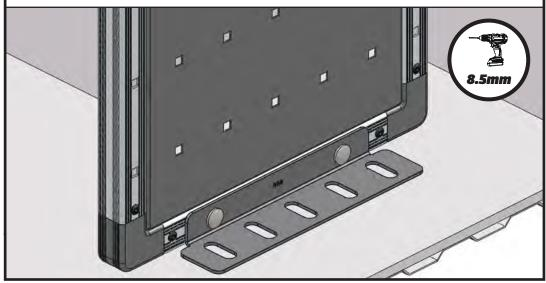
2.8 Bolt down through the floor brackets using M8x50 hex bolts and M8 washers, secure under the vehicle using M8 washers and M8 nyloc nuts.
