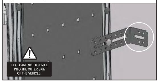
3.6 Secure the fixing brackets to the side of the vehicle using M6x14 hex bolts, M6 washers and M6 flange nuts.
