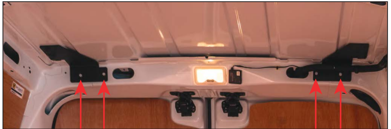
M6 1/4 TURN NUT INSERT LOCATIONS
