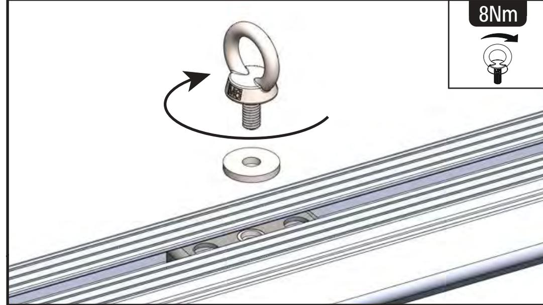
**3** If the eye bolt is removed from the roof bar remember to also remove the rail plate. The rail plate must not be left inside the roof bar when it's not in use.
