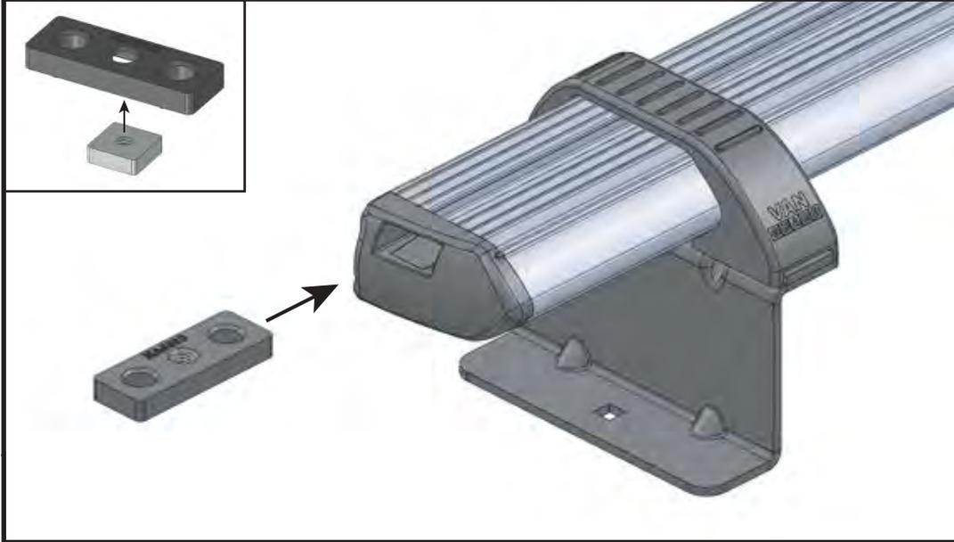
**2** Place the eye bolts onto the roof bars and secure to the the rail plates positioned in the t-track.
